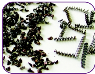
Swarf produced by DNMG-442-CT Insert
