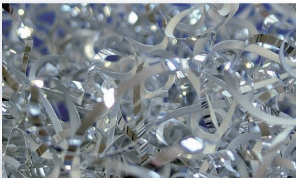
Without 3D-chip breaker: Flow chips
