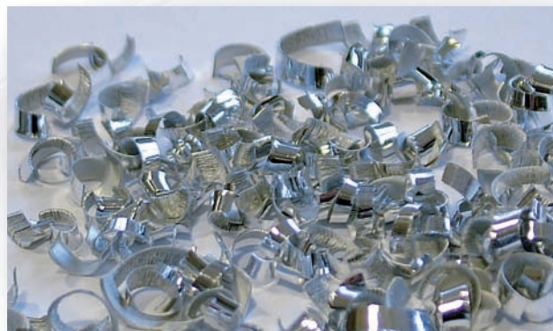
With 3D-chip breaker: Breakage chips
